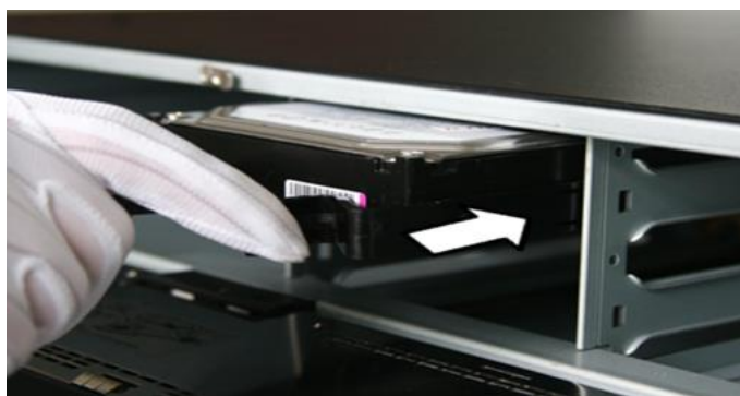
Figure 2-4 Insert Hard Disk
