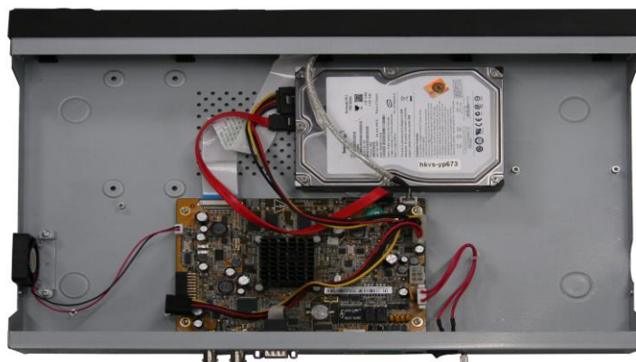
Figure 2-9 Fix Hard Disk
